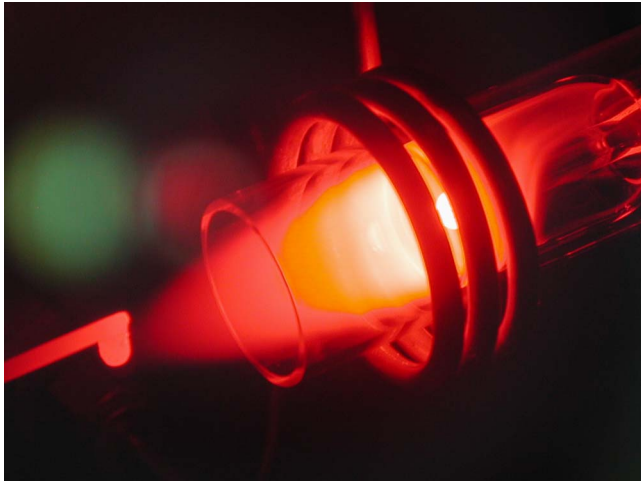
Fig. 3 Axial heating of a copper rod by rf-ICP
